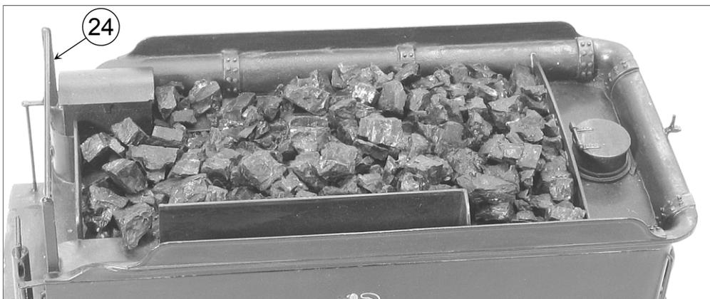
On GER tenders there was a hinged flap or fall plate at the front to prevent coal falling down between floorboards and tender. Solder a length of 0.7mm brass wire into the rebate on the underside of this fall plate (part 20) and then thread two split pins over this wire and into the two holes in the tender front. You should be able to get at the shanks of the split pins with your soldering iron from inside the tender body to spot solder them. This should then give you a hinged fall plate.
