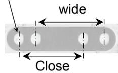
The tender is coupled to the loco using a coupling bar (part 31) and 8 BA screws screwed into the captive nuts on loco and tender chassis. The screws are not tightened fully so that the bar is free to pivot. The coupling bar has pairs of holes at different centres to allow close and wide coupling depending on the curves on your layout.
