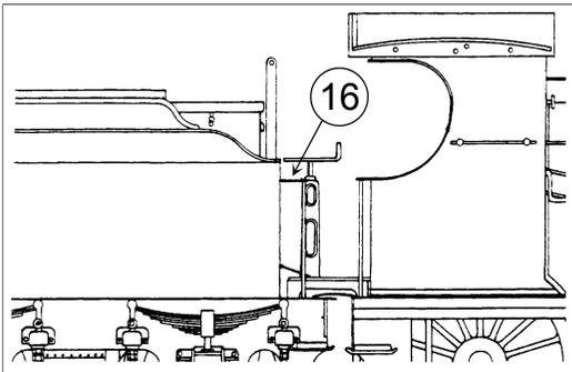
A number of J15's had a lower cab cut out and the tender handrails were correspondingly lower to match up with the cab. This was mainly on the early built locos but check photos. If you are modelling one of these locos part 16 will require folding through 90° and soldering to the tender front. The cab side has the cut out marked with a etched line so use this to set height.
